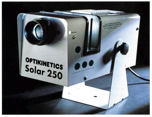
Optikinetics Solar 250, the world's most popular Effects Projector, has been produced since 1973. The projector is fitted with a Xenophot 250W M33 lamp which has a light output of 1200 lumens at lens. European safety requirements, new technology and casing modifications have been incorporated to improve the projector for the end user.
